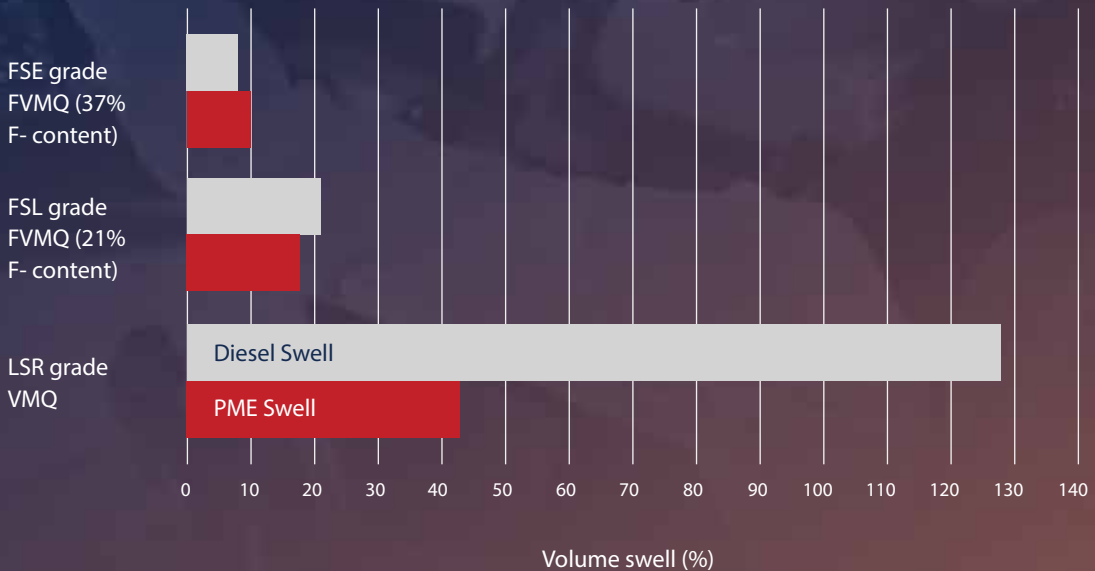
Immersion test in Diesel and PME 72 h at 120°C
